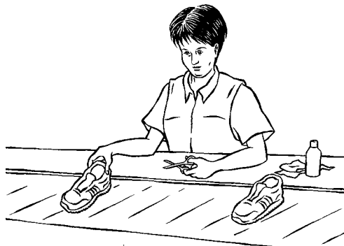
A conveyor belt at arm's length reduces the need to reach.
