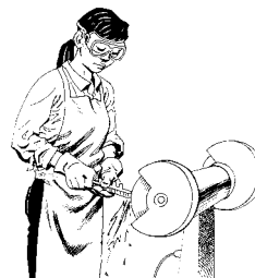
Grinding cast metal parts creates silica dust.
